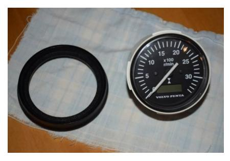
2. Rotate the outer ring counter-clockwise from the tachometer unit.
