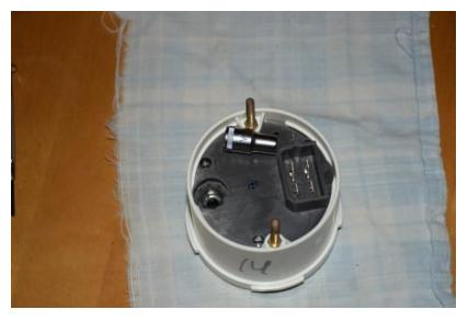
3. Now it's time to remove the tachometer from the white plastic holder. Use 6 mm socket to loose the 2 brass-nuts and. Move the back core unit slightly and then press out the black core unit from the white bracket.
