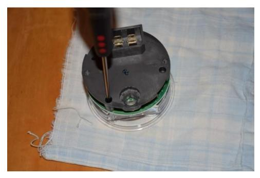
5. Swap the Tachometer side again. Remove the screws by a screwdrive
