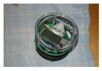
8. Now when the new LCD is in place check the cable again that it's securely fixed into place. Then remove the LCD outer protection film.
