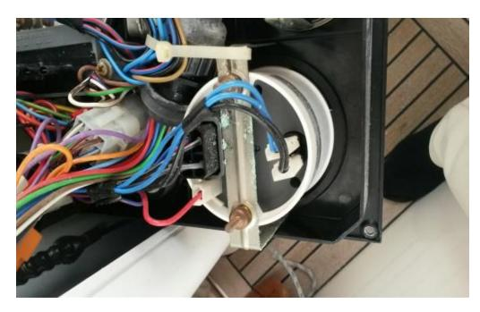
1.Detach the tacho from the dashboard by the 2 brass-nuts holding the bracket. Pull the taco forward until you have it in your hand.
